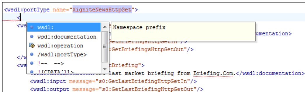
Figure 236: Namespace Prefixes in the Content Completion Assistant
