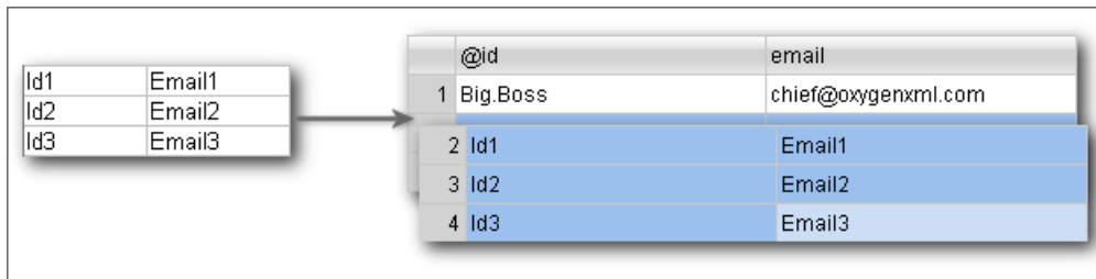
Figure 8.9. Copying tab separated values into grid
