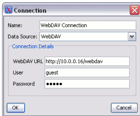
Figure 13.21. The WebDAV Connection Configuration Dialog
