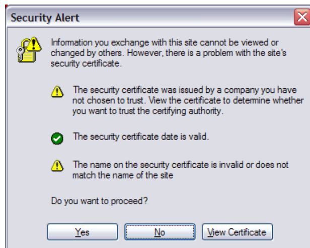
Figure 4.14. Security alert - untrusted certificate
