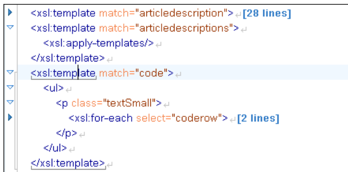
Figure 4.37. Folding of the XML Elements
